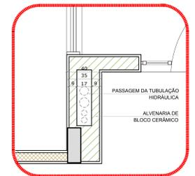
**5** DETALHE - SHAFT HIDRÁULICA
